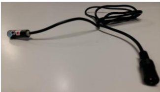
Figure 6: Laser diode with 0.5 mW output at wavelength of 650 nm (Class II).
