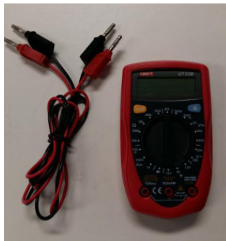
Figure 5: Digital multi-meter and wires with banana connectors
