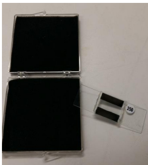
Figure 6: Sample box and one Ti-coated Fabry-Perot (FP) etalon (for illustration purpose, the sample number in this figure is #250)
