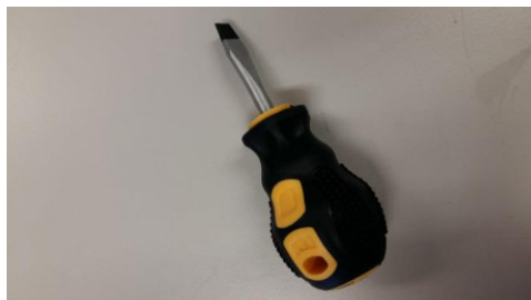
Figure 7: Flat-head screw driver for adjusting the beam size of the laser diode
