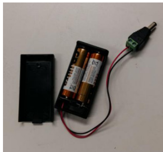
Figure 3: Battery pack with 2 \times 1.5\text{V} AA batteries and outlet plug for the laser diode
