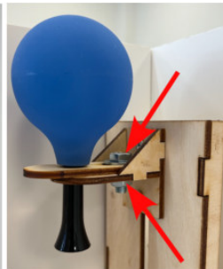
Figure 4: The two wingnuts on the back can easily be loosened to allow the release mechanism to slide vertically. Also, the vertical nut can be used to enable horizontal adjustment.
